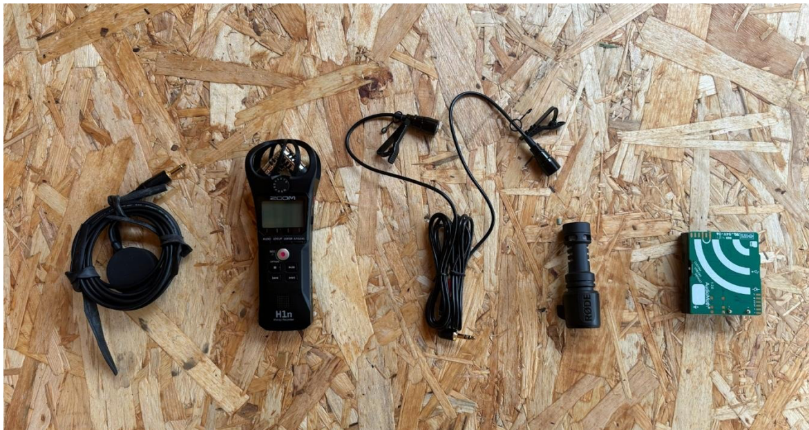
Figure 4 Recording devices included (from the left): a contact microphone, a handheld recorder with built-in stereo microphone, a clippable microphone, a directional microphone, and a full-spectrum acoustic logger.
